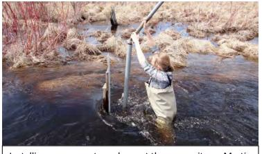
Installing a pressure transducer at the gauge site on Martin
