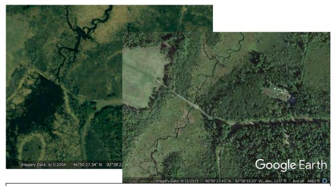
**Figure 35. Aerial photos of Martin Branch at Marshall Rd in 2004 (top) and 2015 (bottom).** A new road crossing has restored stream connectivity and drained a large water impoundment on the upstream side of the road. Photo source: Google Earth.
