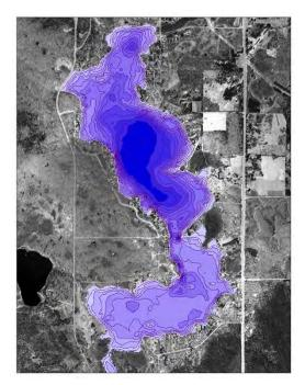
Figure 70. Bathymetric depth map of Big Lake created using the BioSonics echosounder
